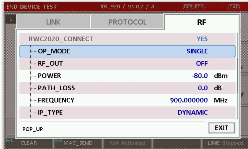
Fig 2.9 Single-tone Mode Control in RWC5020A
