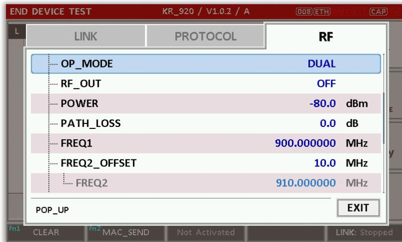
Fig 2.11 Dual-tone Mode Control in RWC5020A
