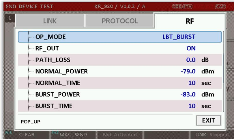
Fig 2.7 LBT Burst Mode Control in RWC5020A
